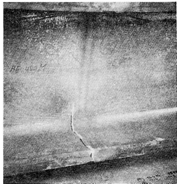
Fig. 9 Fracture of the butt welded specimens without holes
