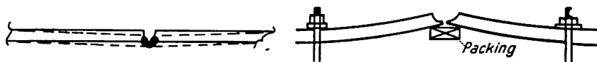
Distortion of Flange Due To Welding From Top Only. Flange Glanded Down About 18" Back From Each Side of Weld.
