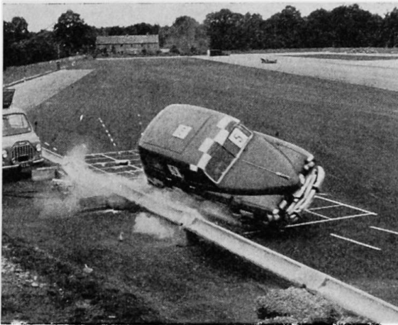
Fig. 8. Impact with D. A. V. concrete guard rail at 46 mile/h and 20 deg.
