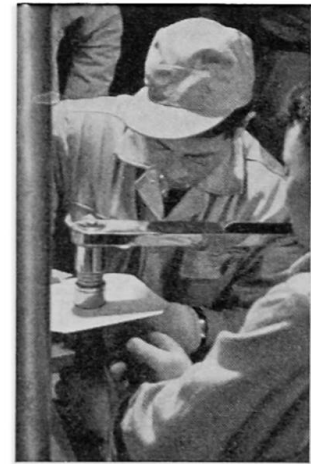
Fig. 10. Bolt tightening test by use of load cell.
