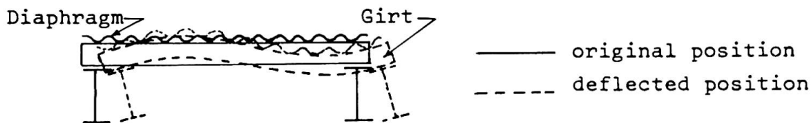
Fig. 4 Columns with Diaphragm-Girt Bracing
