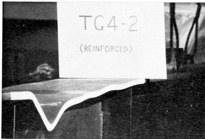
FIGURE 9 VIEW OF COMPRESSION FLANGE AFTER COLLAPSE
