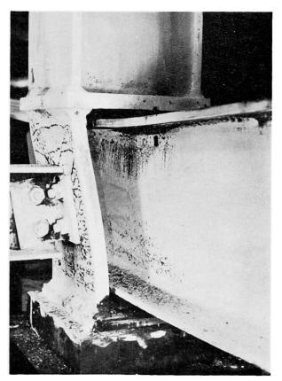
Type 3: The upper box, with no primary nor secondary beam, began to show signs of yielding in the walls at 95 T.
