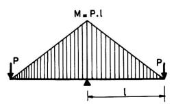
This distance was chosen in order to respect the shear-moment relationship existing at the support of a uniformly loaded continuous beam. A 15 T load acted on the column.
