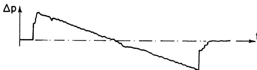
Fig. 1. Pressure signature due to the sonic boom \Delta p = 0 corresponds to atmospheric pressure.
