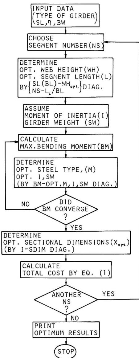
Fig. 7. Flow Chart of the Design Procedures
