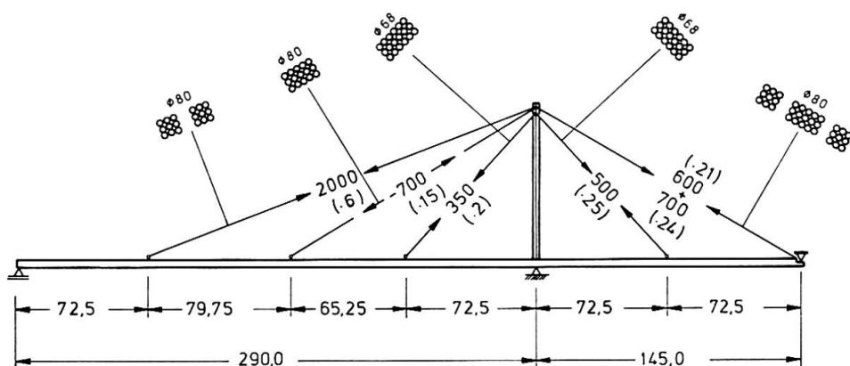
Fig. 2: Cable sections and prestressing:
