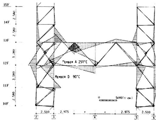
Fig. 4: Distribution of bending moment according to the ordinary design load
