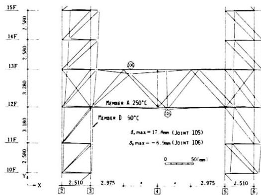
Fig. 3: Joint displacement according to only thermal expansion
