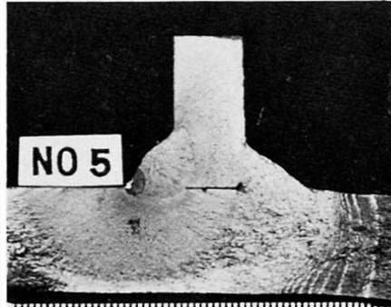
Fig. 5 Fracture surface (from under-cut)
