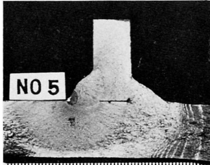
Fig. 5 Fracture surface (from under-cut)
