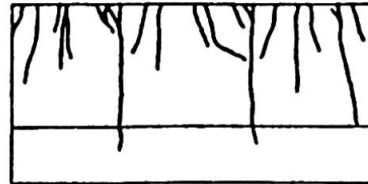
Fig. 3(b) Crack pattern development of A-2-0 (no skin reinforcement)
