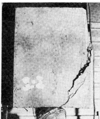
Fig. 12 Test set-up for laboratory-made push-out tests
