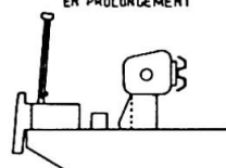
GARDE - CORPS + BARRIERE PRECONTRAINTE TYPE "BAGNOLET"
