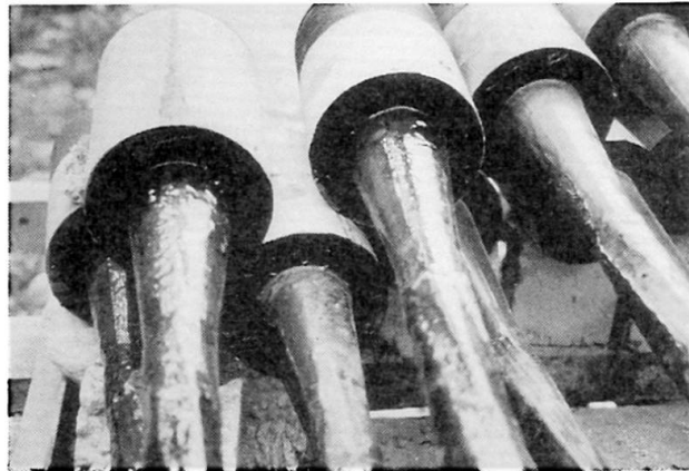
Fig. 5 Finished Sockets after Casting
