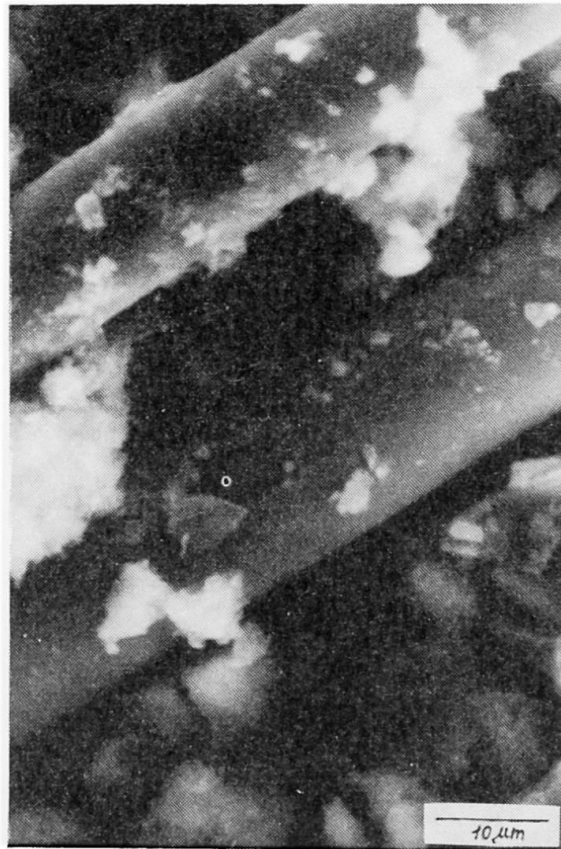
Fig.5 SEM of ESAP fibres in the cement matrix /360 days, water curing, fibres: 4.4%/
