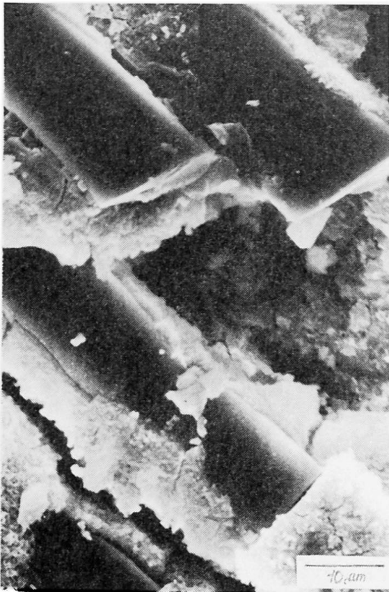
Fig. 4 SEM of REZAL fibres in the cement matrix /360 days, water curing, fibres: 4.4%/
