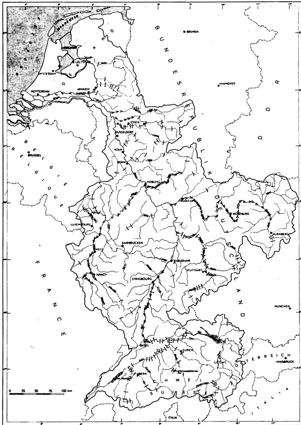
fig.5 Overview of the most important dams with locks and reservoirs in the Rhine catchment area. These constructions have primarily been put into place in order to better regulate the river's water levels and to evenly distribute water drainage throughout the year.
