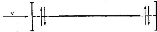
Fig. 28. Open Slots in Bridge Deck Yield Aerodynamically Stable Section. This feature Now Adopted in the Design or Reconstruction of All Large Suspension Bridges.
