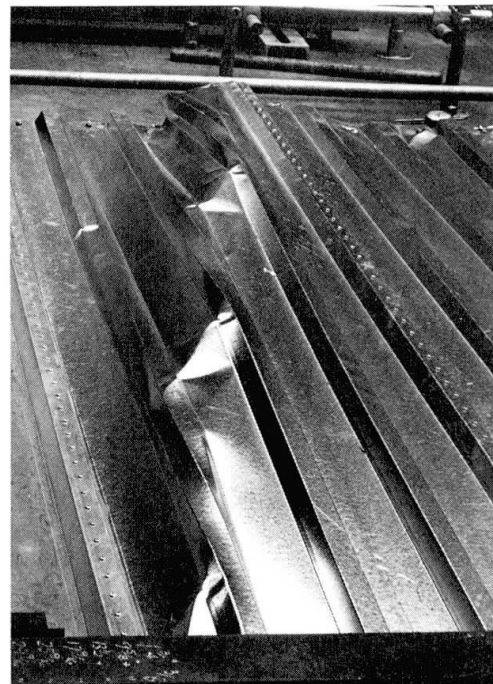
Fig. 11. Illustrating Overall Buckling Following Fastener Failure – Test 9.
