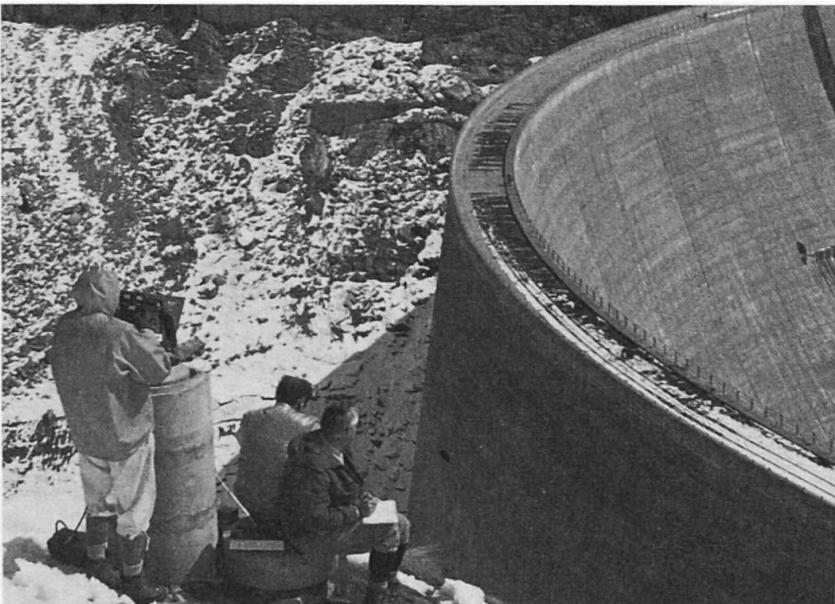
The Mekometer used for dam control measurements
