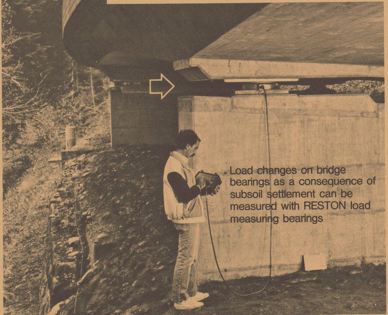
Load changes on bridge bearings as a consequence of subsoil settlement can be measured with RESTON load measuring bearings
