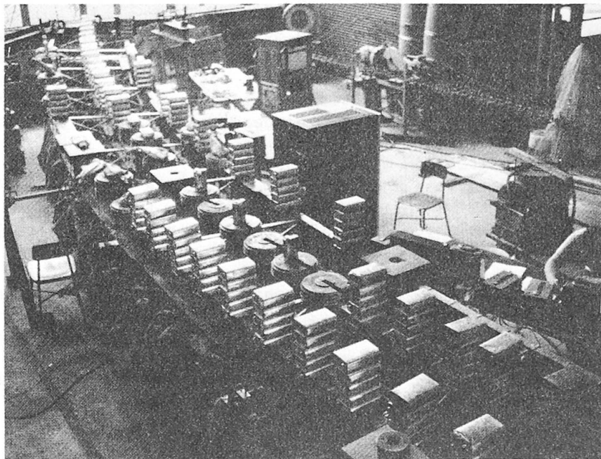
Fig. 3 Dead Loading on Small Scale Seekonk River Bridge
