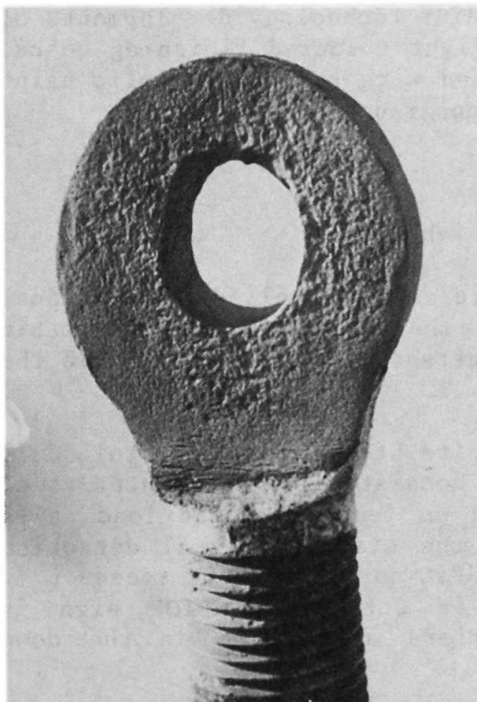
Fig. 5 Wear in suspension rod eye
