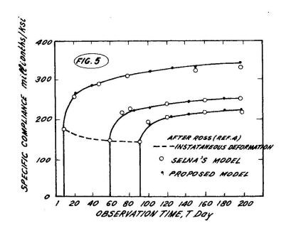
Where TS (K,T) is the total amount the specific creep curve loaded at an age K and temperature T needs to be shifted to fit the reference creep curve.
