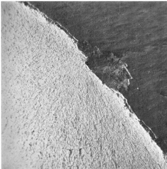
Fig. 4 steel III a, "micro-alloy" Local superficial defect in mill scale, initiation at medium stress:
