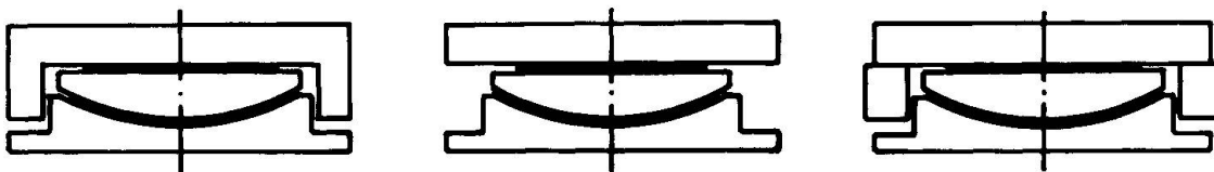
Fig. 4 Spherical Bearing - fixed, multidirectional and unidirectional
