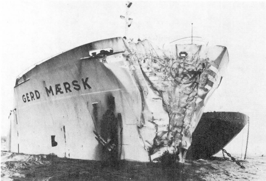
Fig. 2. Collision damage to tanker.
