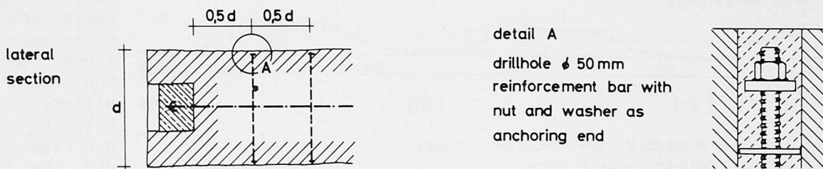
Fig.15 reinforcement rods in the zone of force introduction through prestressing bars
