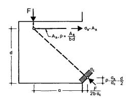
Fig. 4: Simple strut-and-tie model
