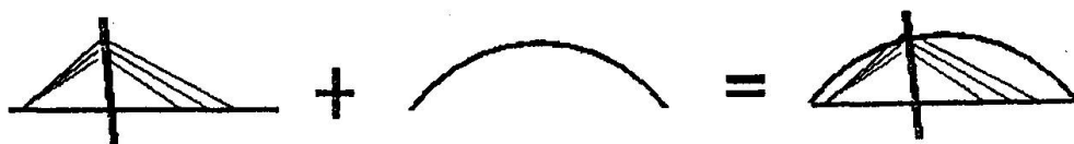
Fig. 9 A new bridge type by adding an arc to a cable-stayed bridge
