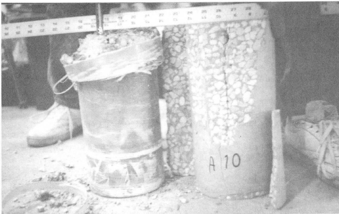
Fig.4 Control and Composite Specimens after Failure
