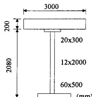
Fig.1 Cross Section
