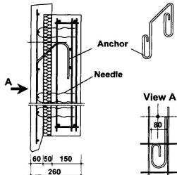
Fig. 1: Structure of the external wall - type WBS 70 in cross section
