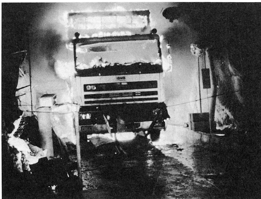
Fig. 3 Fire test on a heavy good vehicle loaded with 2 t of modern furniture
