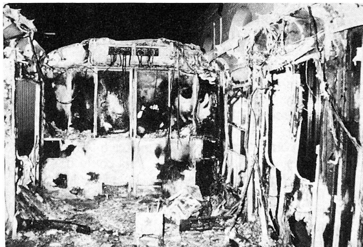
Fig. 2c Aluminium body; fire accident on April 8, 1980, on the Hamburg urban commuter system
