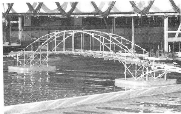
Photo. 3 In-wave elastic model experiment (Scale: 1/40)
