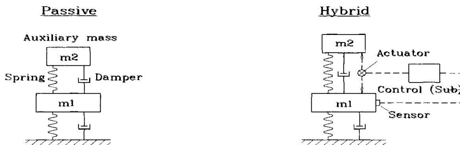
Fig. 6 : Tuned mass dampers
