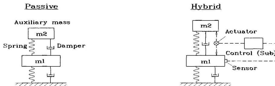
Fig. 6 : Tuned mass dampers
