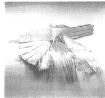
Fig. 1 Pultruded section showing glass reinforcement
