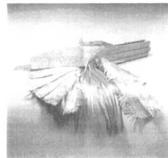
Fig. 1 Pultruded section showing glass reinforcement
