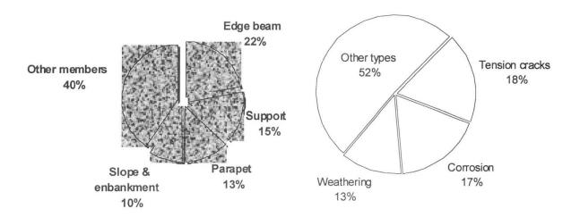
*Fig. 5 Percentage distribution of the damage types remarks on the bridges' different structural members, all condition classes.*
