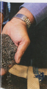
Reusable materials, such as copper, aluminium and even gold, are sorted out from the clinders of waste incineration plants
