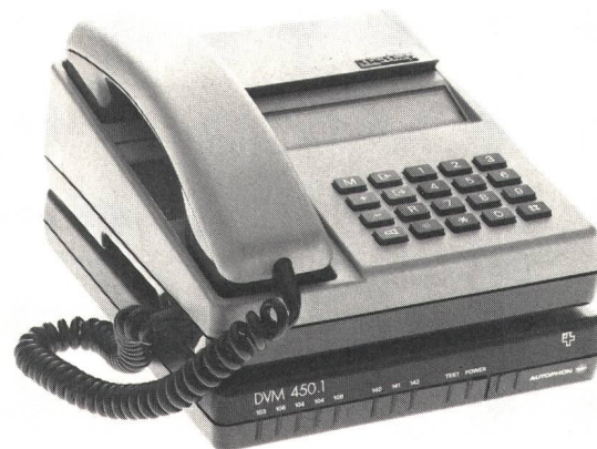
Fig. 6 DOV subscriber device including telephone set
