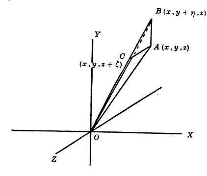
Flow across  $ABC = \eta \zeta \left( \frac{\partial^2 \Psi}{\partial z \, \partial \eta} - \frac{\partial^2 \Psi}{\partial \eta \, \partial \zeta} \right) + \text{terms of degree 3 or more}$ in  $\eta$ ,  $\zeta$ . Hence, dividing by  $\frac{1}{2}\eta\zeta$  and proceeding to the limit  $\eta$ ,  $\zeta \to 0$ , we have  $\left( \partial^2 \Psi - \partial^2 \Psi \right)$
