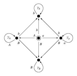
The central state is the start state. Any missing directed edges lead to a dead end failure state.
