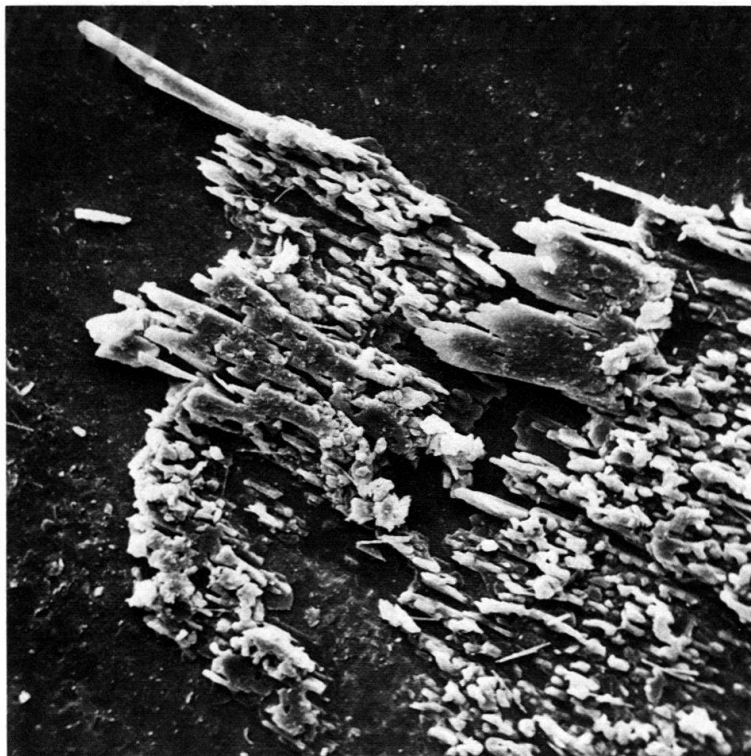
Fig. 6. SEM of gypsum lining on shear plane in mudstone, specimen 349 W (see Fig. 4 und 5, and text). Length of photograph is 0.04 mm.
