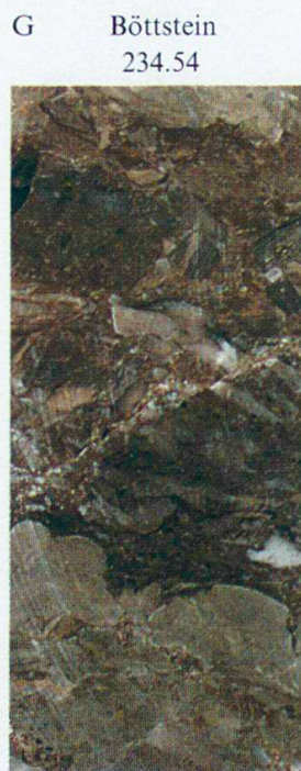
234.74 Erosional surface with well rounded dissolution crust overlain by intraformational conglomerate. Muschelkalk Sulfatschichten III B
