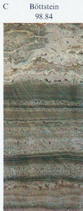
99.06 Clastic gypsum beds and selenite crystals Gipskeuper III B
