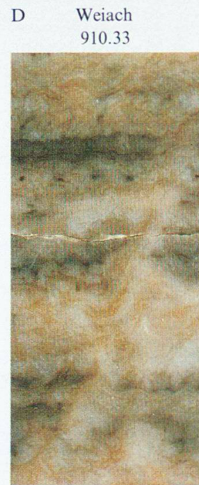
910.53 Anhydrite marker bed containing selenite ghosts and chevron clay bands. Muschelkalk Sulfatschichten III A
