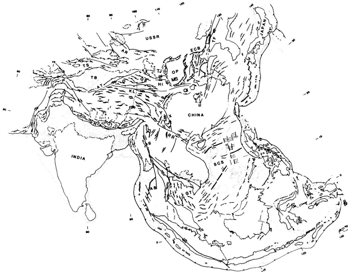
Fig. 5. Generalized Cenozoic tectonic map of southeast Asia. Dotted areas are basins of late Cenozoic deposition. Horizontal arrows indicate sense of slip on strike-slip faults, barbed lines indicate thrust faults in the continental areas and subduction zones in the oceanic areas with barbs on the upper plate, and ticked lines indicate normal faults. Lunate areas in the Tibetan plateau indicate folds, black where Cenozoic, and open where age is unknown but probably Cenozoic. Double lines indicate spreading centers in the South China Sea (32–17 Ma), Okinawa through (Active) and Andaman Sea (Active). Dashed lines in the South China Sea are trends of magnetic anomalies. Dotted line is 1 km isobath in oceanic areas. Compare position of major faults with suture boundaries in Figure 2. ARGAND (1924) recognized that Eurasia absorbed more deformation than India during Cenozoic convergence because it had been deformed more recently than India, and that deformation within Eurasia was unevenly partitioned because of the inhomogeneity of the Eurasian crust. Dotted line in the eastern part of the Tibetan plateau locates the British/Chinese transect. AR = Altai Range; AS = Andaman Sea; AT = Altyn Tagh fault; ECB = East China basins; GT = Gulf of Thailand; H = Himalaya; HI = Haiyuan fault; KL = Kun Lun fault; LS = Longmen Shan; MS = Madong Shan; OP = Ordos plateau; P = Pamirs; Q = Qaidam basin; QS = Qilian Shan; QI = Qinling Mountains; RR = Red River fault zone; S = Sagaing fault zone; TB = Tarim basin; TF = Tan Lu fault zone; TJ = Tianjin Shan; TS = Tien Shan; X = Xianshuihe fault; Y = western Yunnan.
