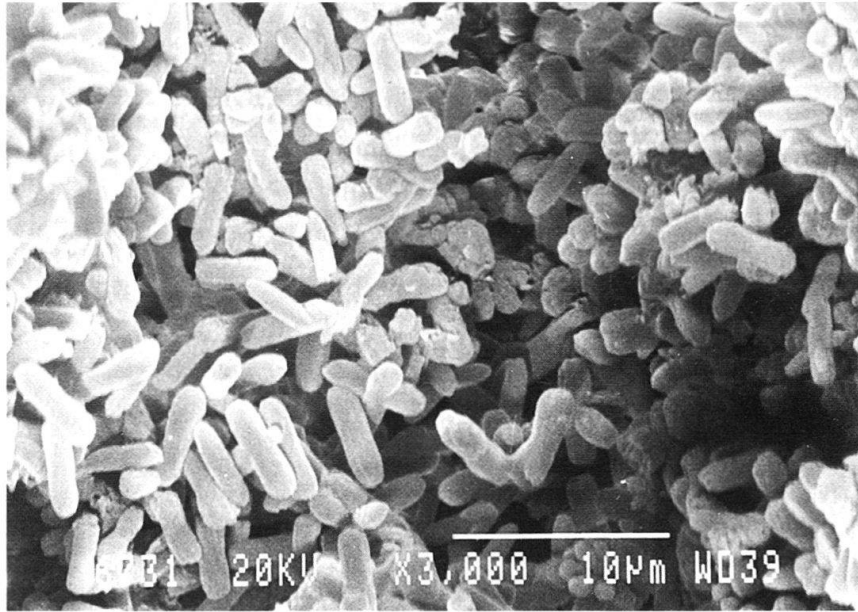
Fig. 16. Matrix of a pristine phosphate layer from the Triassic Bravaisberget Formation of Spitsbergen. Densely packed apatite particles imply a rapid phosphate precipitation event that produced a very high concentration of nuclei in the original porosity of an organic-rich sediment. The particles show rod-like shapes and are made of apatite without any clearly defined crystalline form. SEM photomicrograph. Photo by K.P. Krajewski.
