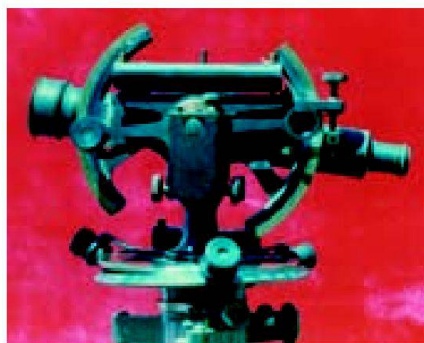
Fig. 5: Everest pattern theodolite designed by for use on revenue surveys.
