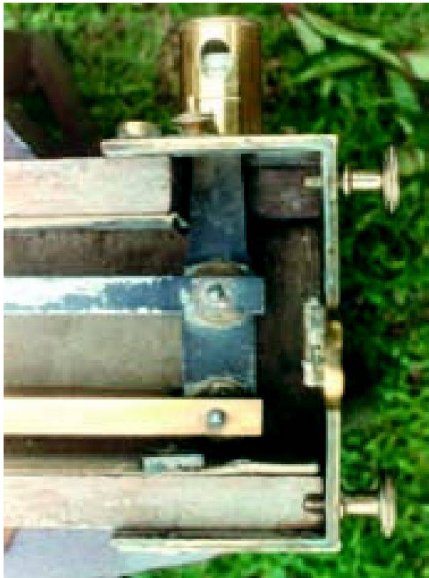
Fig. 4: The end of a Colby bar showing the two bars of different metal joined together in the arrangement to reduce the effect of temperature.
