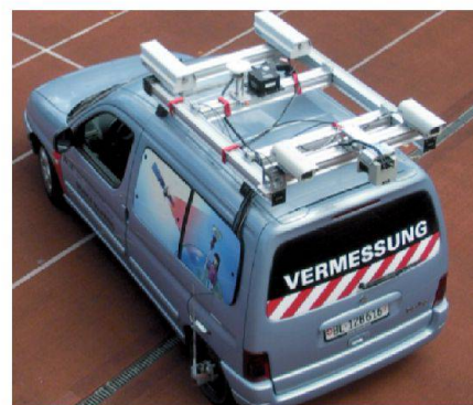
Abb. 1: IVGI Mobile Mapping System.
